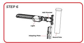
**STEP 6)** Same as round pole installation, please remember to use the adapting plate for round pole installation.
