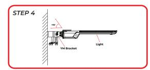
**STEP 4)** Connect the fixture to the bracket and tighten the screws; connect the wires properly and put them into junction box.
