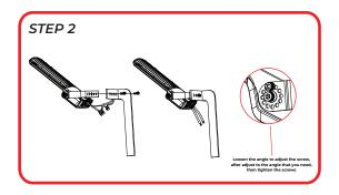
**STEP 2)** Install the mount to the fixture, tighten the mount and install the screws. Connect the fixture to the bracket and tighten the screws; connect the wires properly and put them into junction box.
