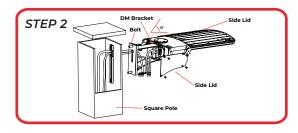
**STEP 2)** Fix the DM bracket to the square pole with bolt, open the side lid of DM bracket, pull the wire into junction box, and connect the wires correctly.
