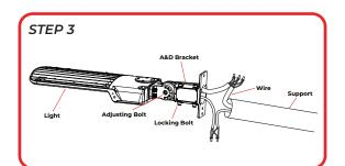
**STEP 3)** Loosen the four bolts on A&D bracket ,connect the wires correctly, and pull the wires into the pole , Place the bracket into the pole and lock the four bots.
